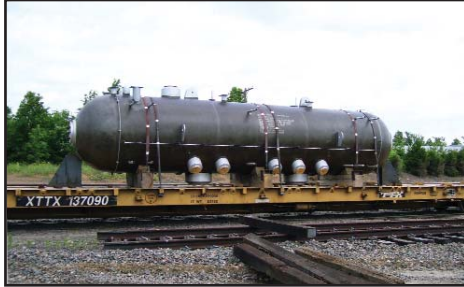
Pressure Vessels (Steam Drum)
