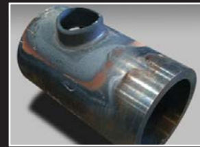
A pulled AG-80 outlet prior to final finishing
