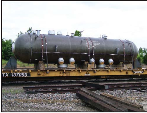
Pressure Vessels (Steam Drum)
