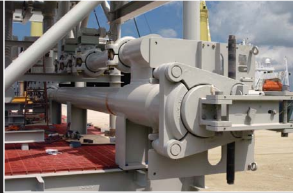
AG-80 Launcher and traps for platform service
