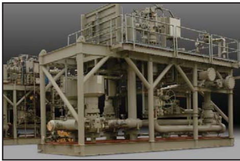
12,000 psi Y-70/Y-80 Scraper Trap Skid
