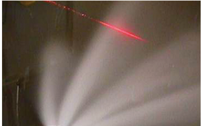
RJM's ultra low NO x oil burner on a test rig showing fuel rich and fuel-lean regions.
