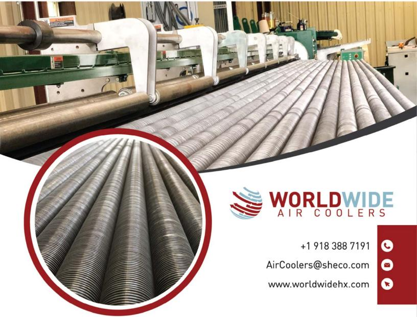
Worldwide Air Coolers announces the addition of the McElroy's latest generation Fintube machine to our growing line of capabilities. With this addition, our capacity has increased to allow us to begin offering fintube parts sales. Worldwide Air Coolers can offer both L-Foot (Wrap-On) and Imbedded (Grooved Fin) finning to meet retube and turn-around needs.
