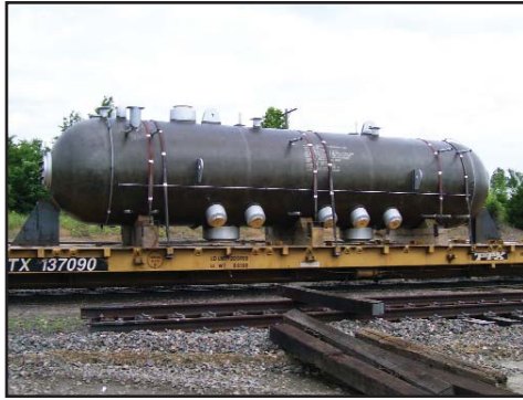
Pressure Vessels (Steam Drum)
